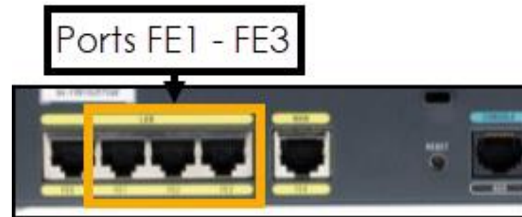
Cisco 857 - Port FE1 (ideal), port FE2 or port FE3
